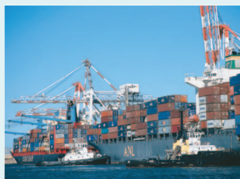
A relatively deep draft and the use of Dynamic Underkeel Clearance ® enables Fremantle's Inner Harbour to handle the larger container vessels.
