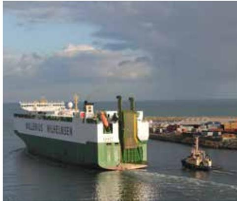
RoRo (roll on-roll off) ships transport a wide range of break-bulk (non-containerised) cargo.
