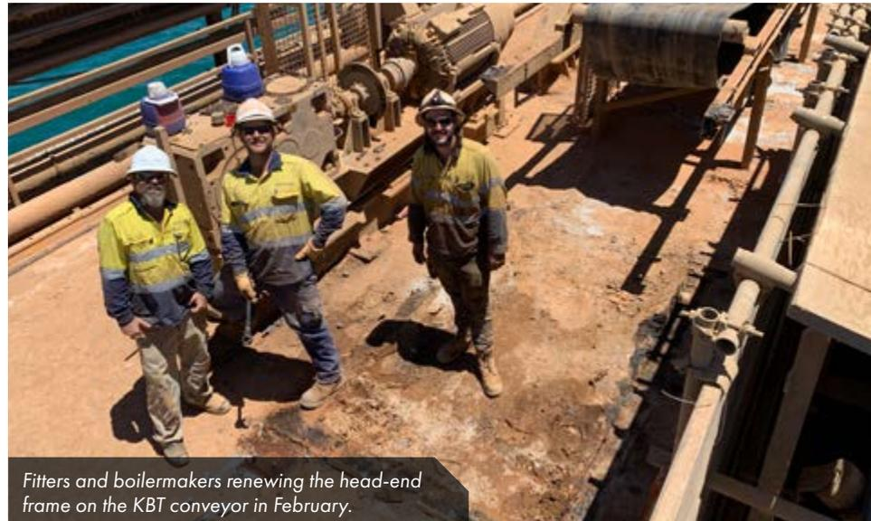
Fitters and boilermakers renewing the head-end frame on the KBT conveyor in February.
