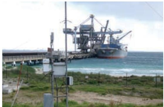
*One of four real-time dust monitors installed at the Kwinana Bulk Terminal.*
