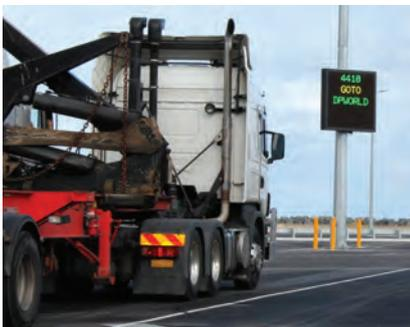
Variable messaging signs are in use to provide directions for trucks in normal and congestion conditions.
