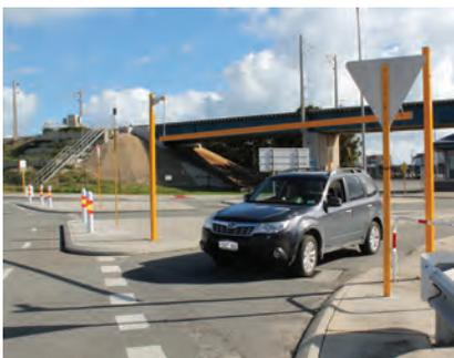
The height restriction bar installed at Gate 3, Victoria Quay is proving effective in reducing truck traffic at the lower end of East Street.
