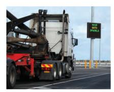
Variable messaging signs are in use to provide directions for trucks in normal and congestion conditions.
