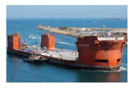
The world's biggest semi-submersible vessel Gavea Lifter, with a deadweight of 50,000 tonnes, arrived at Fremantle on 14 February 2014 for lay-up and survey work. The giant lifter has been used as a temporary wharf at the Australian Marine Complex at Henderson.
