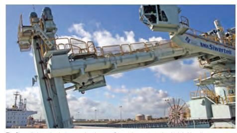
The Siwertell ship unloader is an enclosed system from pick up point in the ship's hold to the transport point, minimising spillage and dust.
