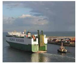
RoRo (roll on-roll off) ships transport a wide range of break-bulk (non-containerised) cargo.
