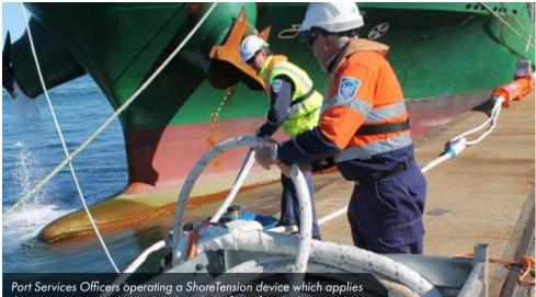
the same constant tension on a ship's lines, for safety and security.
