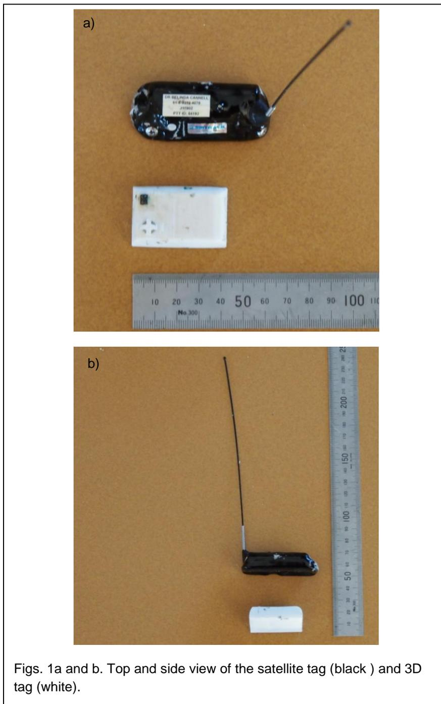
Figs. 1a and b. Top and side view of the satellite tag (black ) and 3D tag (white).
