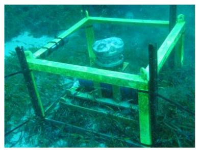
A typical AWAC. (1.0m x1.0m x0.5m high) frame secured to the seabed with star pickets and two anchors
