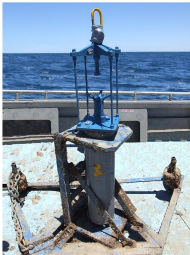
Seabed frame current and wave measuring devices.
