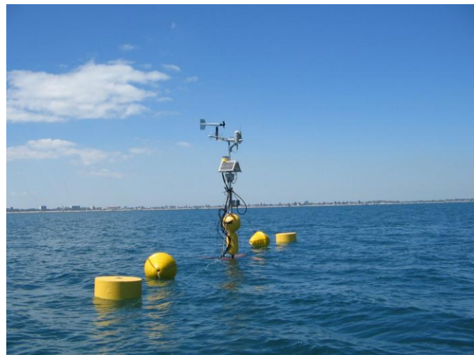
Surface sensor and surface buoys
